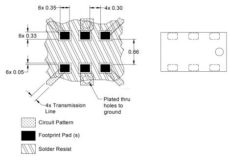
Dimensions are in Millimeters Mounting Footprint
